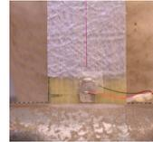
(c) PZT actuator bonded at the root of the beam
