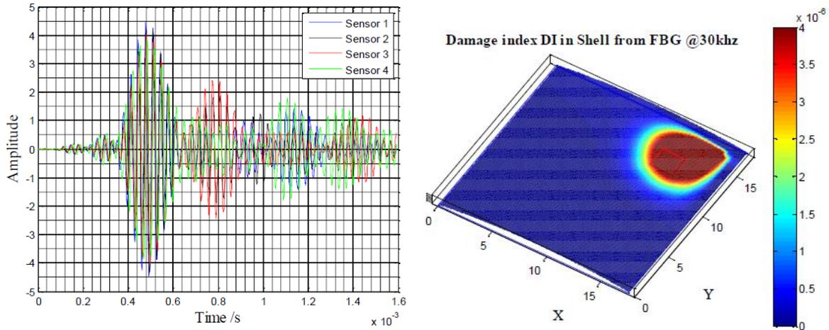
Figure 16 (a) Response signals from 4 FBG sensors at the 4 corners of a curved composite plate with excitation frequency of 30 kHz. (b) Damage Index (DI) in the composite plate deduced from time-of-flight Lamb wave measurements provided by the 4 FBGs.
