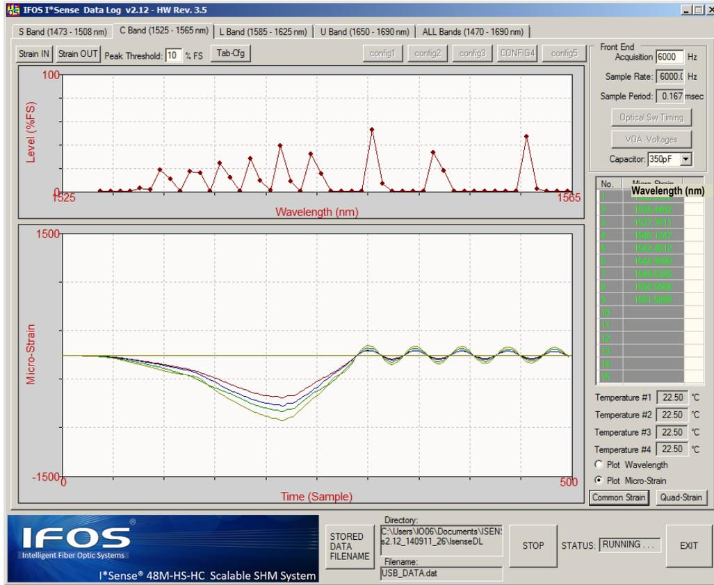
Figure 10: GUI showing a single switch state (C-band for cantilever recording at 6 kS/s) with strain for four of the sensors in the lower plot plotted live at a decimated rate.
