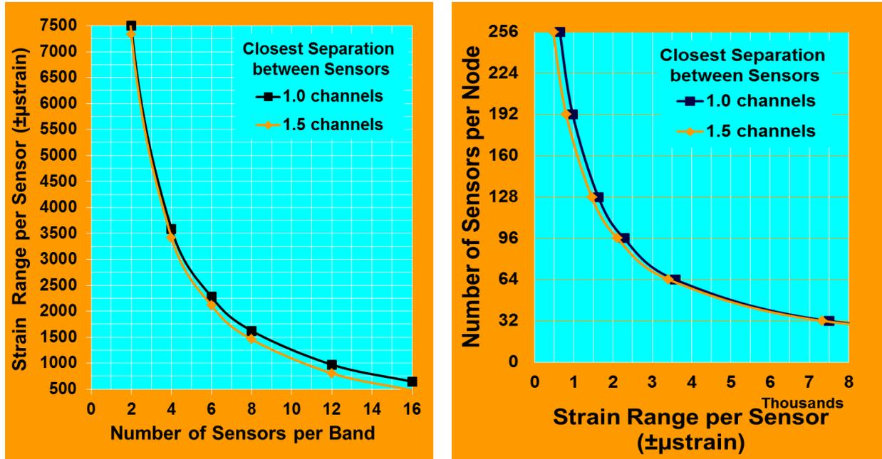
Figure 3: Number of sensors supported dependent on strain range given when each wavelength band is divided into 48 channels separated by approximately 0.8 nm: (a)  $\pm$  strain range per sensor as a function of number of sensors per wavelength band. (b) Number of sensors per interrogation node as a function of  $\pm$  strain range per sensor.
