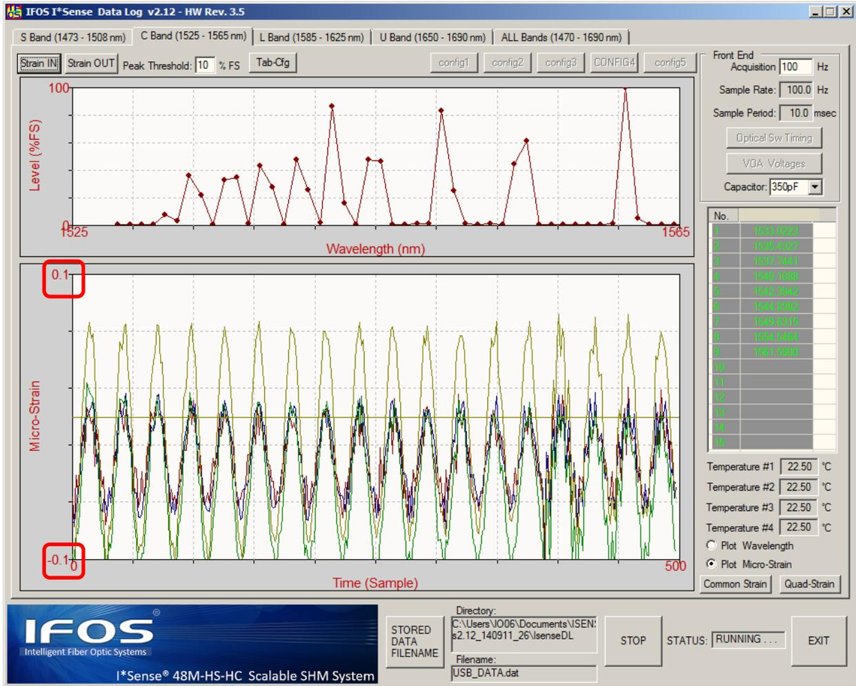
Figure 13: Strain resolution is better than 0.1 microstrain as shown with the cantilever oscillating with a very small amplitude (scale  $\pm 0.1$  microstrain).
