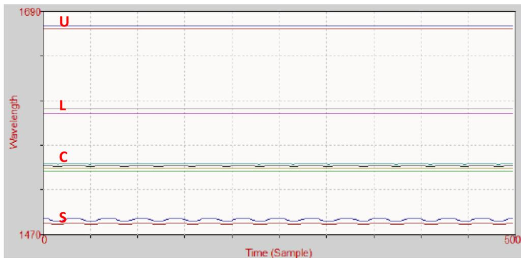
Figure 7: All band wavelength response for a large (>15") deflection of the cantilever beam end.
