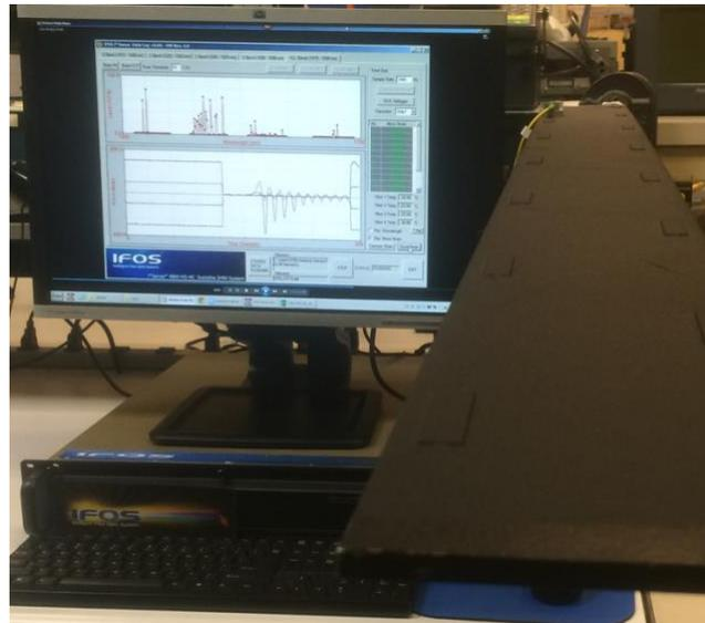
Figure 5: Interrogator (left) and cantilever beam (right).
