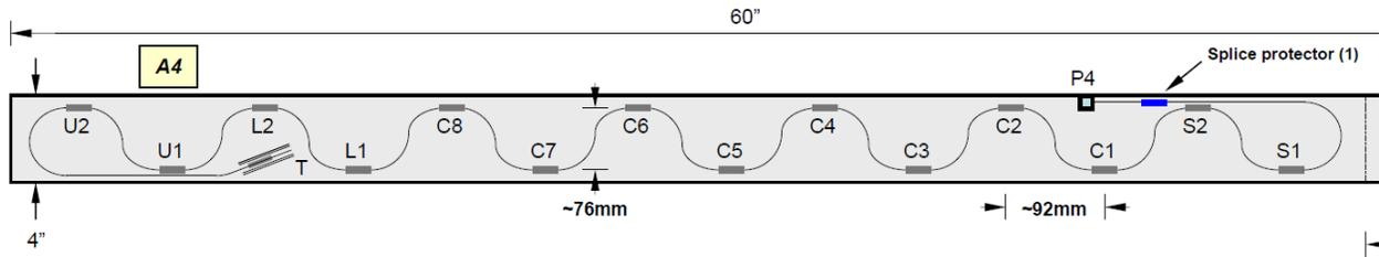
Figure 4: Design layout for sensors on cantilever beam.
