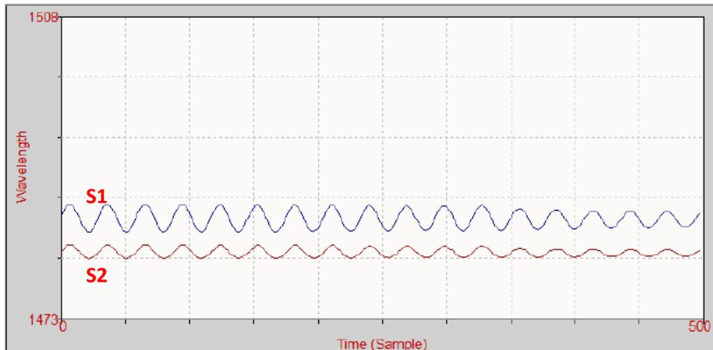
Figure 8: S band wavelength response for a large (>12'') deflection of the cantilever beam end.
