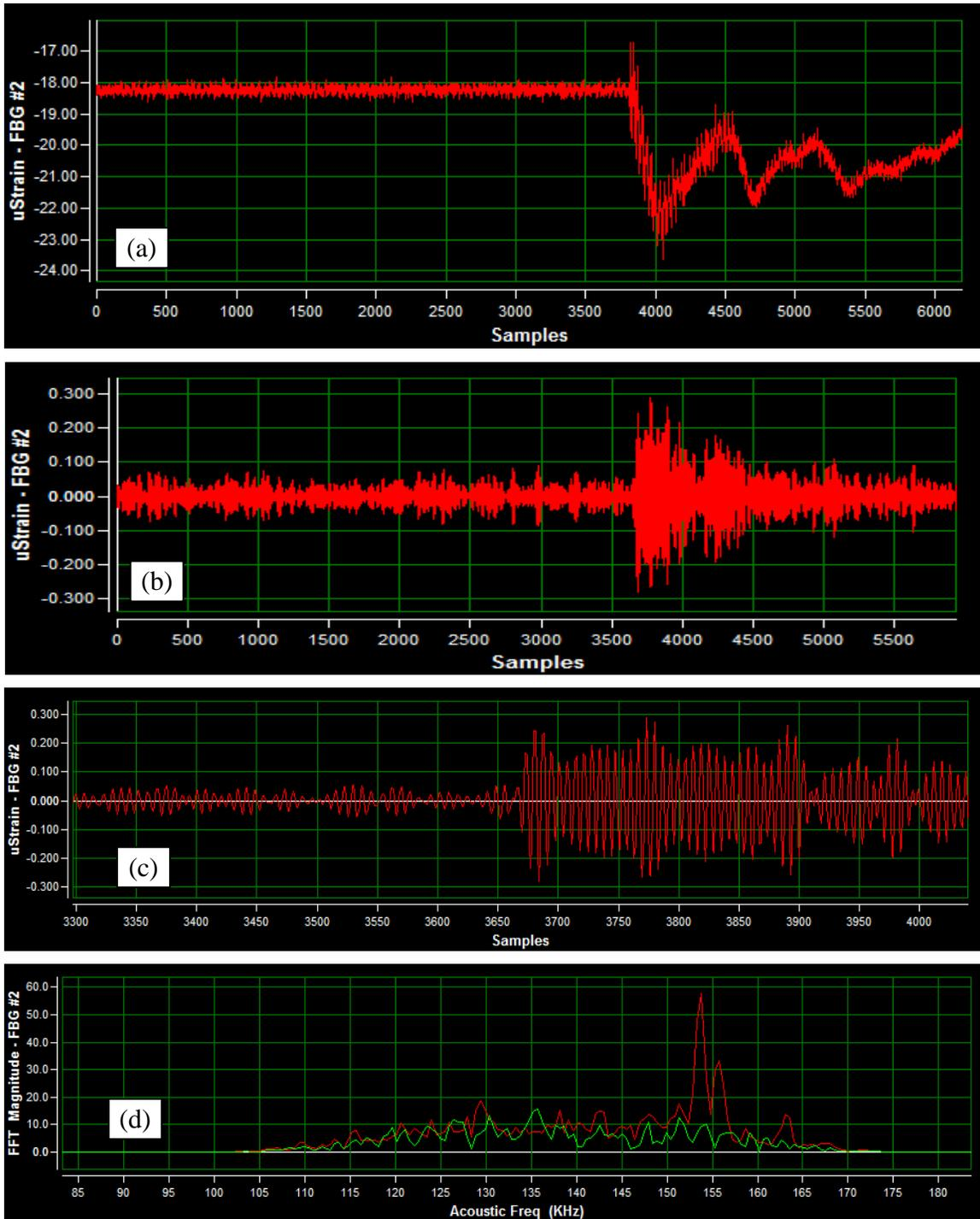
Figure 15: Same as previous figure but (a) unfiltered strain, (b) with application of a bandpass filter between 105 and 170 kHz, (c) time zoom into the region of multiple AE events, (d) comparison of pre-trigger (green) and post-trigger (red) signals in the frequency domain.
