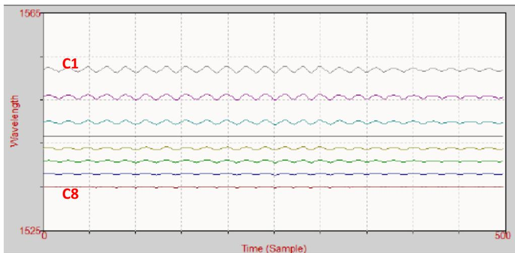
Figure 9: C band wavelength response for a large (>12'') deflection of the cantilever beam end.
