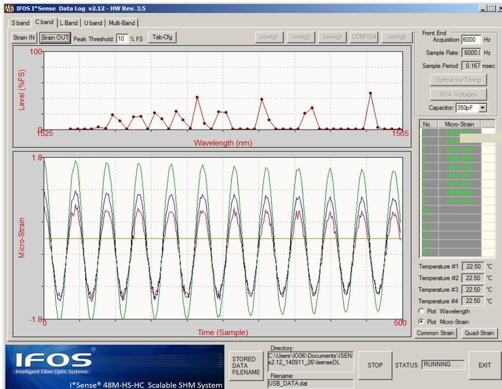
Figure 12: Reasonably clean sinusoidal oscillations of the cantilever are detected down to microstrain levels (scale  $\pm 1.9$  microstrain) when running at full speed (6 kS/s).
