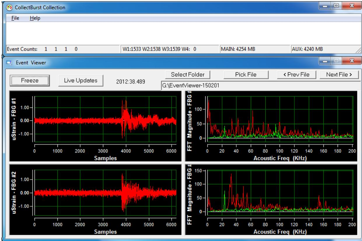
Figure 14: High-speed sampling at 1 MS/s for detection of acoustic emissions (AE) from a pencil led break.
