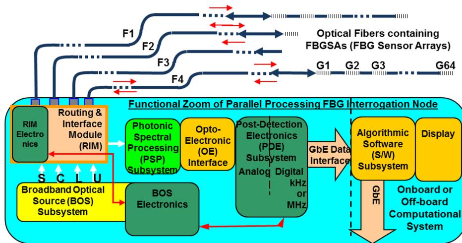
Figure 2: Functional schematic of building block interrogation node including photonic, electronic and software/firmware subsystems and modules.
