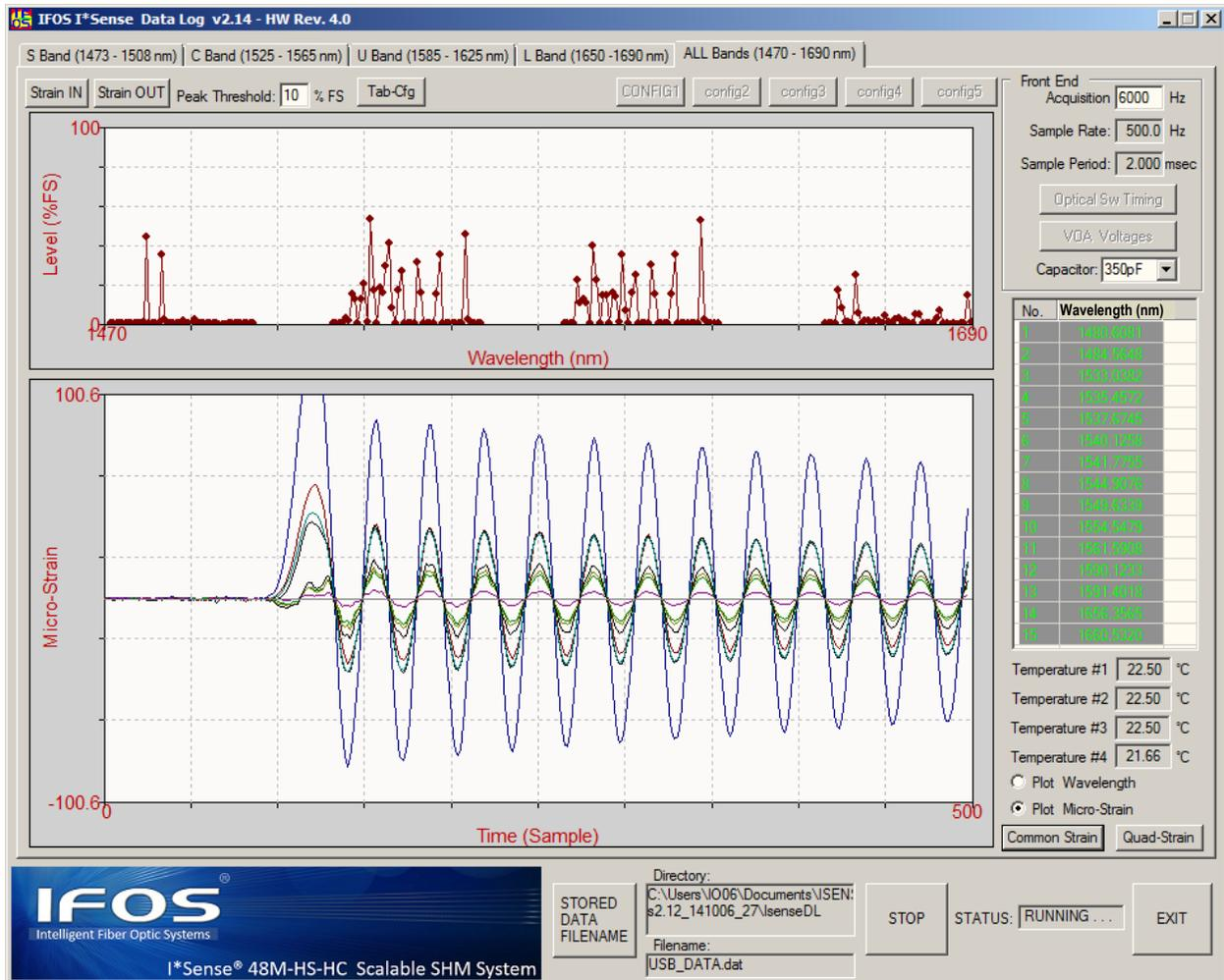
Figure 6: GUI version 2.14 showing strain variation for multiple FBGs on the cantilever beam of the previous section
