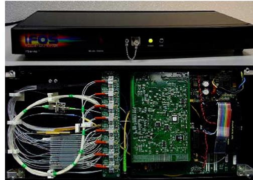
Figure 4. Layout of the 8 channel prototype.
