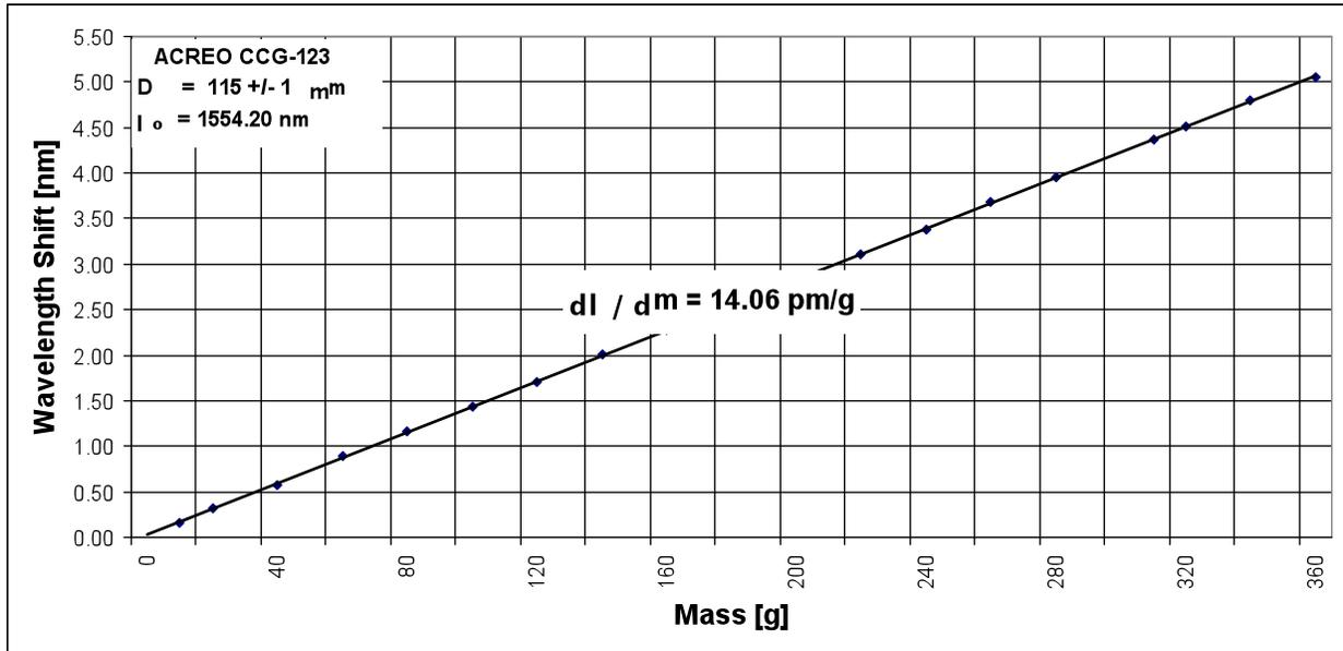
Figure 5. Weight measurement for chemical composition grating from ACREO with room temperature unstrained center wavelength 1554.2 nm.
