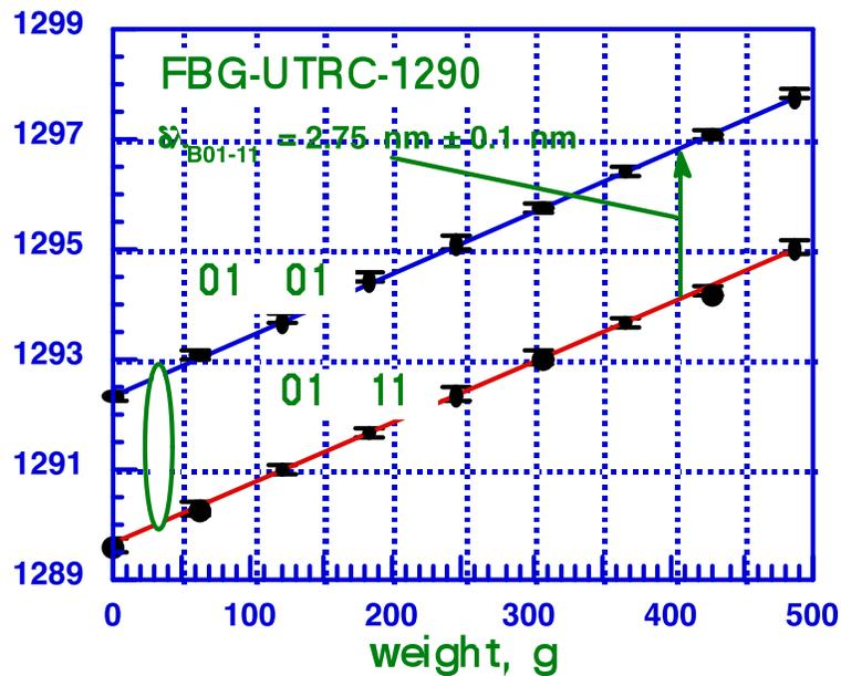
Figure 4. Two-mode fiber grating: Bragg resonance wavelengths as a function of weight applied to the fiber (producing a tension on the order of  $\approx 1\%$  per kg).
