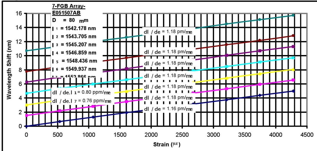
Figure 9. 7-Grating array in 80- $\mu\text{m}$  bend-resistant optical fiber: Wavelength shift versus strain deduced by assuming  $E_{silica} = 73 \text{ GPa}$  and  $g = 9.81 \text{ ms}^{-2}$ .
