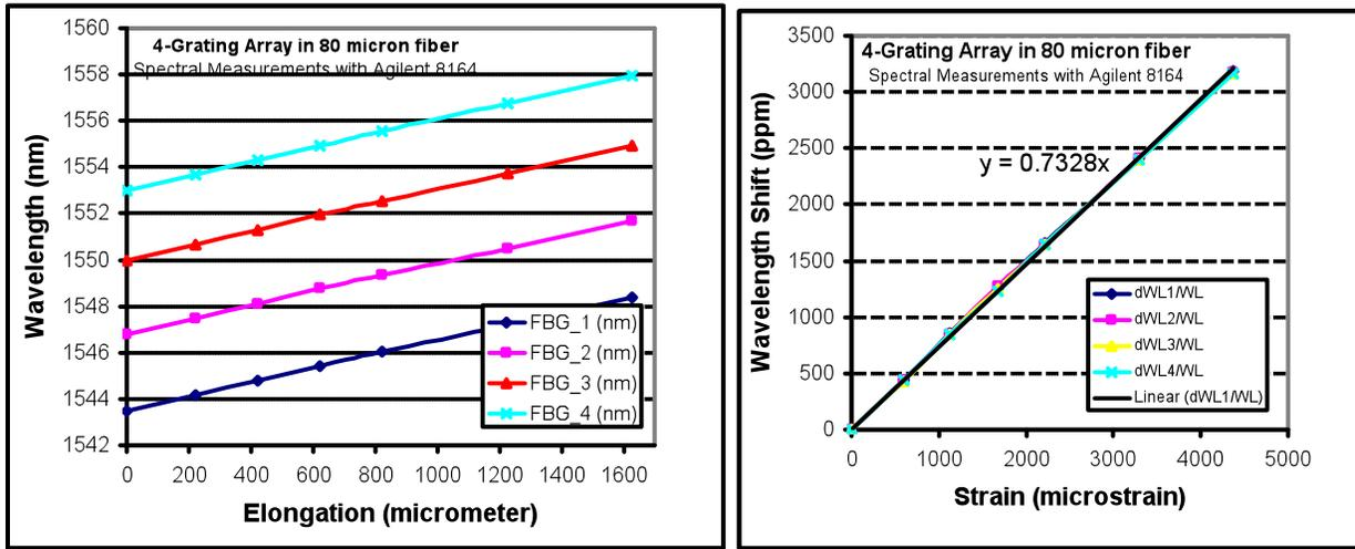
Figure 11. 4-Grating array in 80-um bend-resistant optical fiber: (a) Wavelength shift versus elongation given a separation between clamp points of 371.5 mm. (b) Fractional wavelength shift versus fractional elongation (strain).
