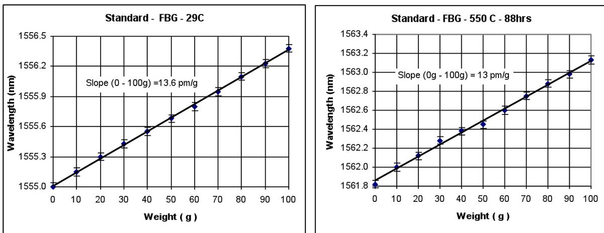
**Figure 3. Standard FBG: Weight measurement (a) at 29°C, and (b) after 88 hours at 550°C (at which temperature the strain dependence was retained although the reflectivity decreased by 10 dB).**
