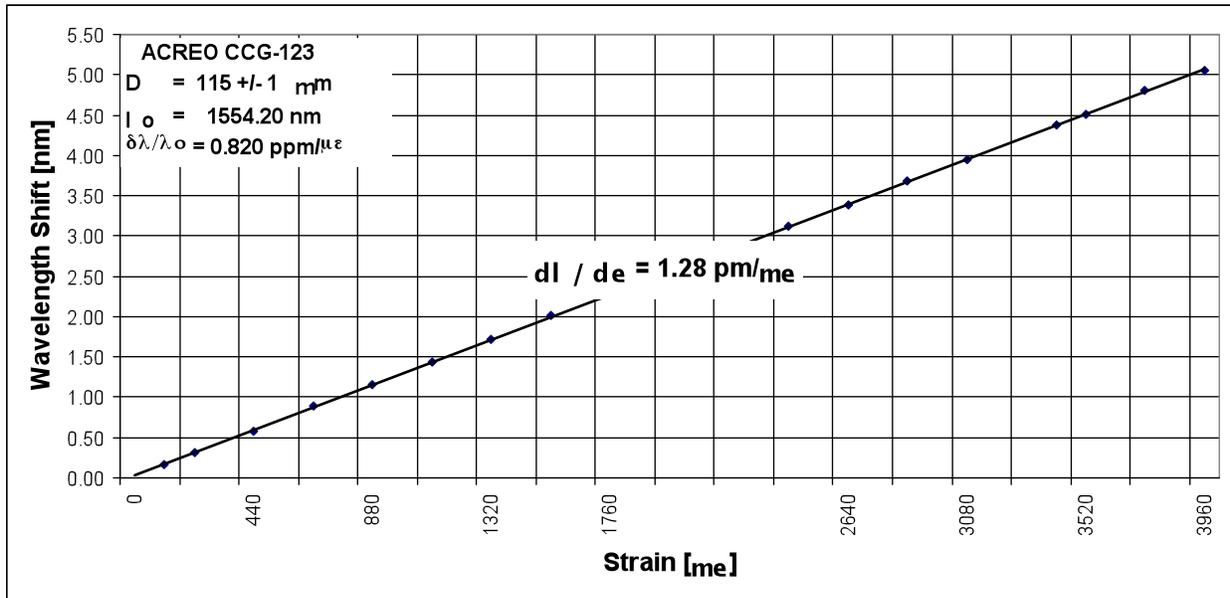
Figure 6. Gage factor deduced from weight measurement for ACREO grating.
