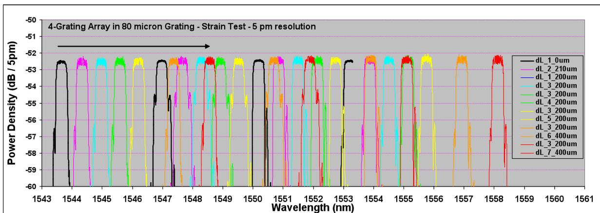
Figure 10. 4-grating array in 80- $\mu\text{m}$  bend-resistant optical fiber: Wavelength spectra seen increasing in wavelength as the grating array is stretched in increments given in the legend.
