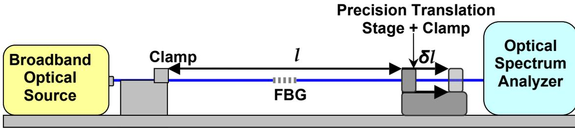
**Figure 2. Stretching Measurement Setup** for calibrated strain tests involving putting tensile strain  $\epsilon = \delta l/l$  on the fiber gratings via stretching an amount  $\delta l$  given initial length  $l$ . The length  $\delta l$  is greatly exaggerated in the schematic – in general it ranges from ppm to less than 0.5%.
