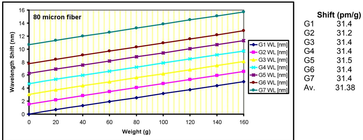
Figure 8. 7-Grating array in 80- $\mu\text{m}$  bend-resistant optical fiber: Wavelength shift versus weight for the Bragg wavelength peaks of the previous figure showing an average shift of 31.38 pm/gram and fractional shift 20.3 ppm/gram.
