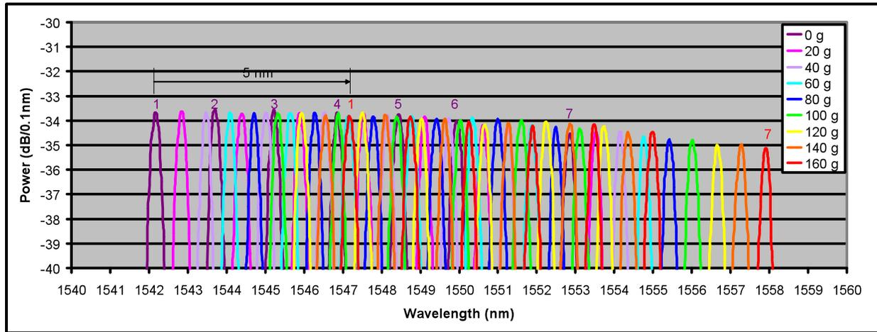
Figure 7. 7-grating array in 80- $\mu\text{m}$  bend-resistant optical fiber: Wavelength spectra for 9 different weights showing shift of approx. 5 nm when tension is applied by hanging 160 grams.
