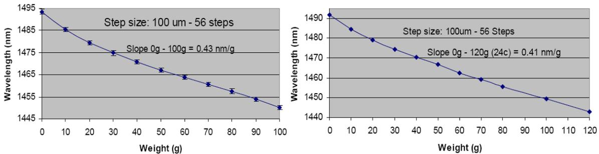
Figure 12. IFOS fabricated electric-arc-written Long-Period Grating (LPG): Weight measurements at (a) room temperature, and (b) at 650°C after being held at that temperature for 32 hours.
