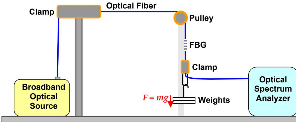
Figure 1. Hanging Weights Measurement Setup for calibrated strain tests involving providing tension on the fiber gratings with hanging weights.
