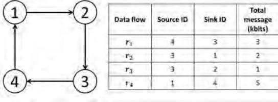
Fig. 4. Four-node ring with four packets to schedule.
