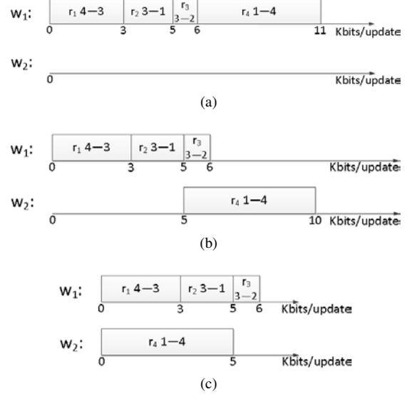
Fig. 5. Frame schedule with different sophistication and resource configuration. (a) Serialized schedule (TTP). (b) Two wavelengths, 1 transceiver at each node. (c) Same as (b) with 1 additional transceiver at nodes 1 and 4.
