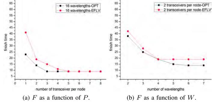
Fig. 9. Comparisons of EFLV and optimum: CDC ROADM model.
