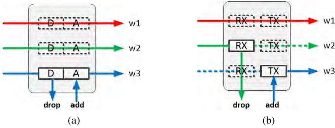
Fig. 2. (a) A/D model, A: add, D: drop; (b) CDC model, TX: transmitter, RX: receiver.
