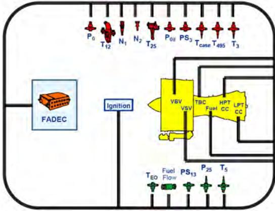
Fig. 1. Aero-engine control with shared communication infrastructure [1].
