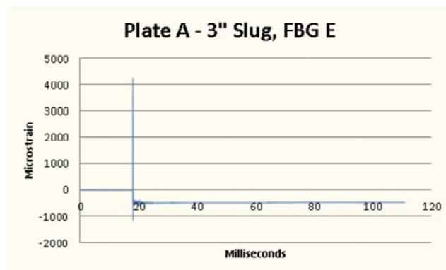
**Figure 10: FBG sensor measurements at location E**
