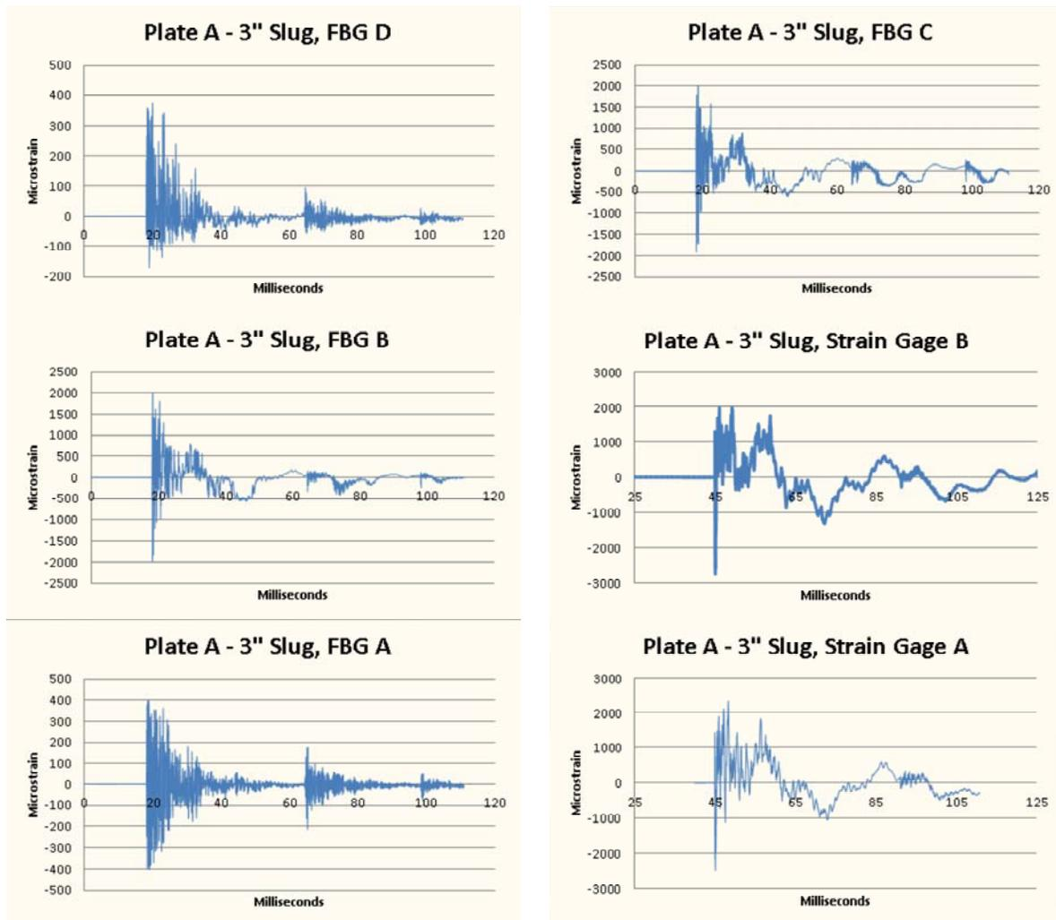
Figure 11: Time history data of strain measurements at location A-D
