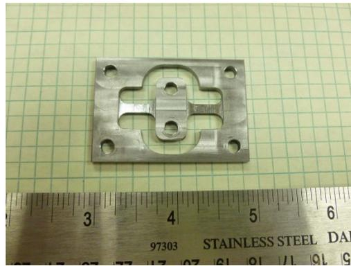
**Figure 5: Single manufactured FBG fixture**
