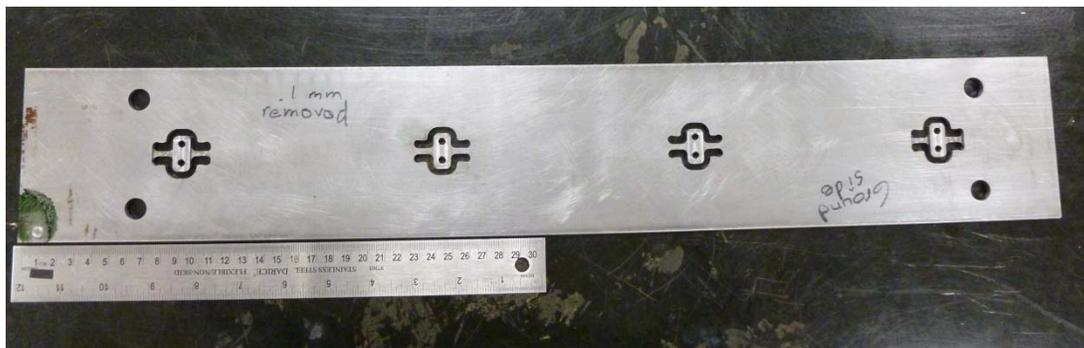
**Figure 6: A plate (Labeled as Test Plate A) with four integrated FBG fixtures**
