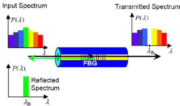
Figure 1: Functional principle of a fiber optic Bragg grating
