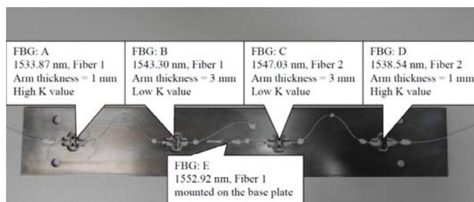
Figure 9: Test plate A with instrumented sensors
