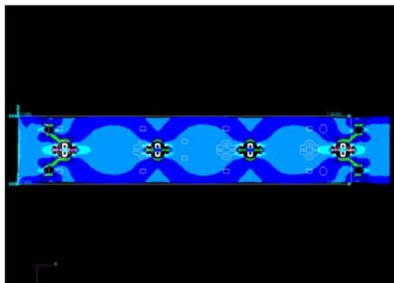
Figure 8: Strain contour for Test Plate A
