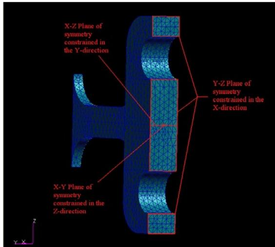
Figure 3 Meshed FBG model showing constraints
