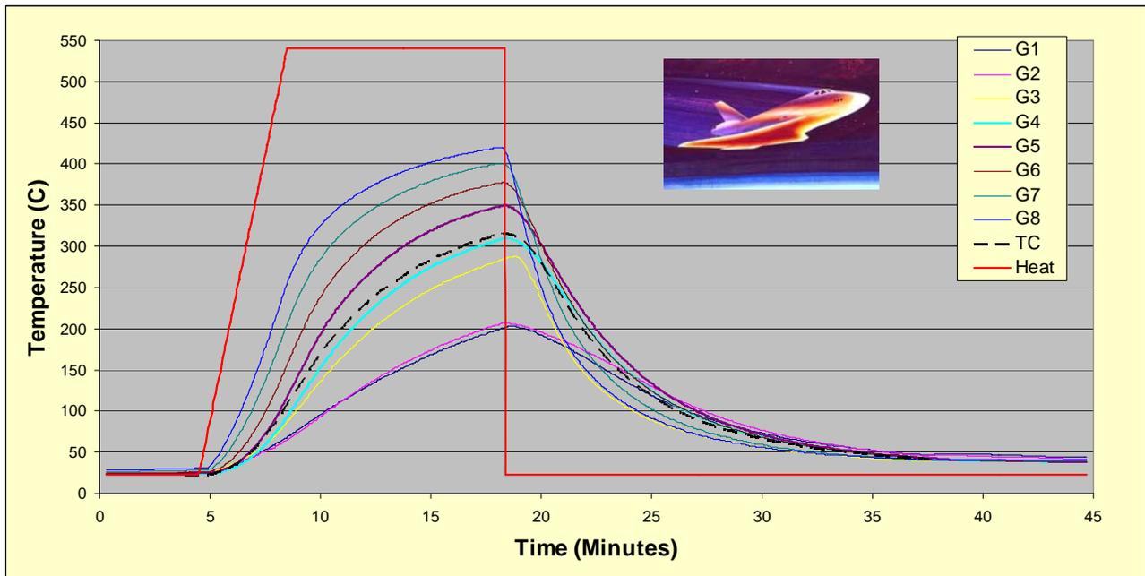
Fig. 6 Temperature profile tracking at different depths in TPS with FBG array (G1...G8) and thermocouple (TC) near G4.
