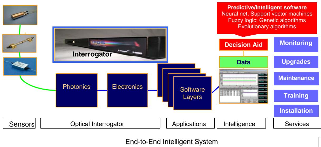
Fig. 1 End-to-end intelligent fiber optic sensor system.
