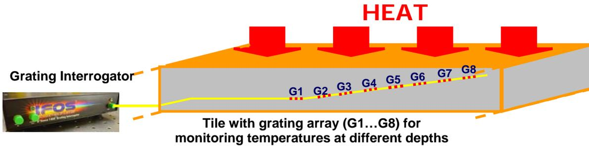
Fig. 5 Setup for measurement of temperature profiles in TPS tiles using an array of fiber Bragg gratings (G1...G8).
