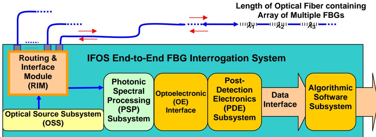
Fig. 3 IFOS parallel processing FBG interrogation supporting multiple FBG arrays.
