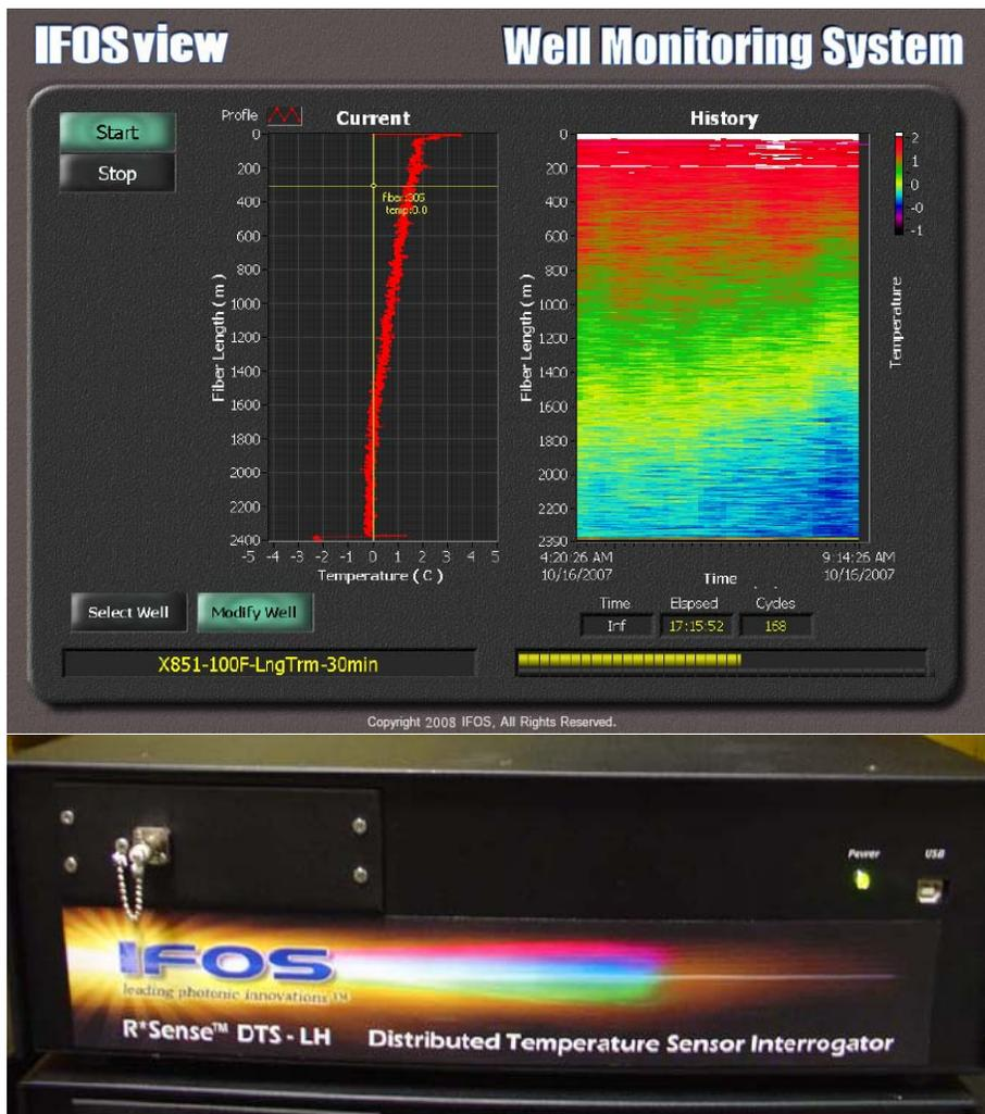
Fig. 4 IFOS DTS system with temperature as a function of distance along an optical fiber cable measured over 2400 meters with 1 meter spatial resolution.
