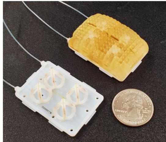
Fig. 1. An FBG-based, multi-axis sensing pad. Tower structures, embedded with FBGs, provide three-axis force information at each structure location. An additional FBG is isolated inside a metal sleeve and provides temperature compensation. The sensing unit is encapsulated inside a urethane elastomer, which serves as the gripping surface. Grooves in the cover decouple signal between the towers.
