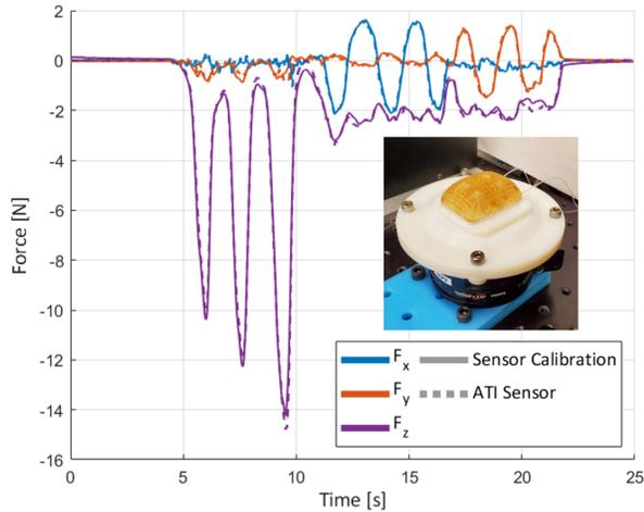
Fig. 5. Sensor calibration of normal and shear forces compared to the ATI, with an  $R^2 = 0.9956$ . Inset is picture of testing setup, with the sensor rigidly mounted on top of the ATI. Forces are applied manually to each taxel, which is also transferred to the ATI below.
