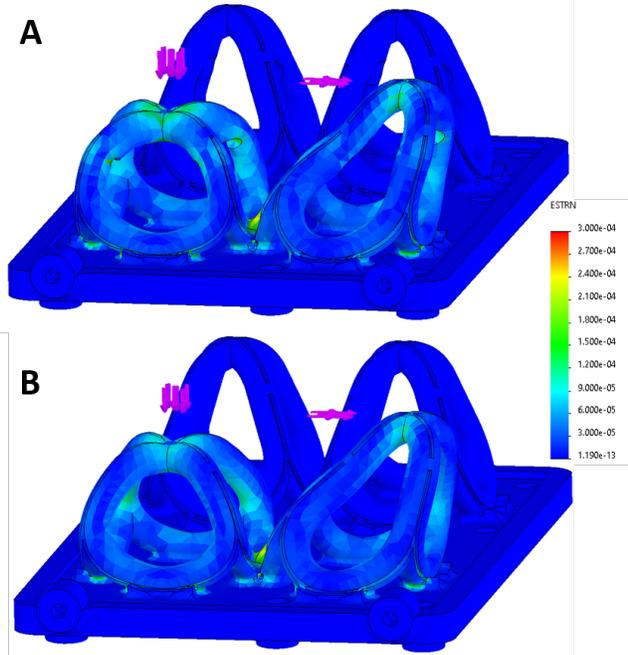
Fig. 3. Finite element analysis. Normal and shear forces are applied to tower structures. (A) The structure includes cutout features in the pillars. (B) Without the cutouts. Significantly more strain is observed at the FBG location in case A. Moreover, tower angle results in a desirable ratio between normal and shear force sensitivity.
